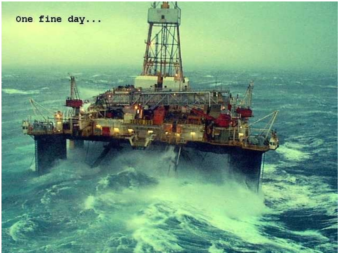
The attached image shows the semi-submersible drilling rig 'Sedco 706' riding over a giant wave in the North Sea at 60°30'N 000°50'E during the winter 2000/01. The deck should have been 60 feet above the water line and the rig is approximately 325 feet wide.
