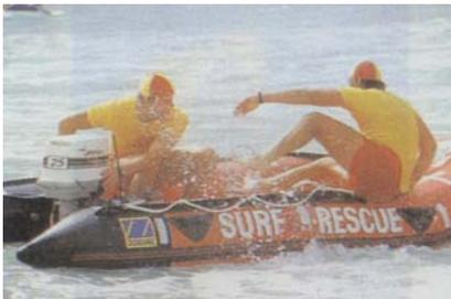
When ready to go, the skipper instructs the crew to board by jumping, hip roll or body roll as the motor's gear is engaged and the duck departs.
