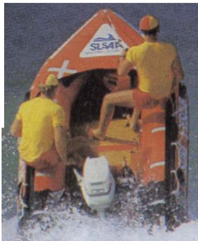
Practice controlled accelerations to bring it up onto the plane by using the crew to lean forward to counteract bow lift.
