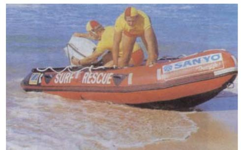
In beach running, a course is taken between the white water along the trough of the swell until a saddle of unbroken green water allows the duck to work to seaward. It negotiates the green water at 30° (to reduce wave face incline) and slows to reduce impact. At the top of the wave, a burst of throttle stops the duck falling into the trough as it simultaneously returns to parallel running and regains the plane. White water must be negotiated at 90°.
