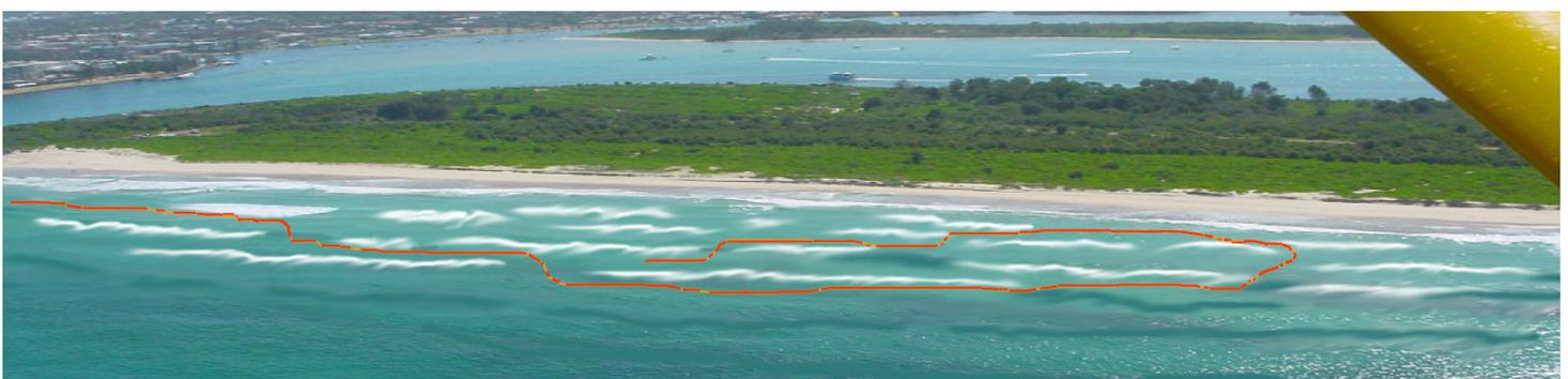
In beach running, a course is taken between the white water along the trough of the swell until a saddle of unbroken green water allows the rib to work to seaward. It negotiates the green water at 30° (to reduce wave face incline) and slows to reduce impact. At the top of the wave, a burst of throttle stops the rib falling into the trough as it simultaneously returns to parallel running and regains the plane. White water must be negotiated at 90°.
