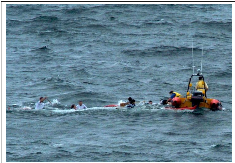
The propellers must be stopped to pick up persons from the water
