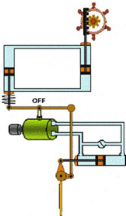
The purpose of the pressure relief valve is to reduce damage to the steering gear if it is hit by a large \_\_\_\_\_.
